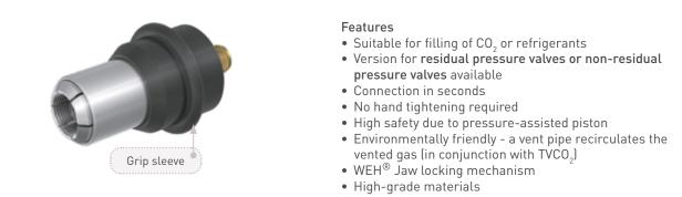
The type TW52 quick connector has been developed especially for filling gas cylinders with gaseous and liquid  $CO_2$  or refrigerants. Connection to the cylinder is made within seconds without tedious screwing and unscrewing, thus preventing RSI resulting in the inflammation of tendons and abrasion of joints.
