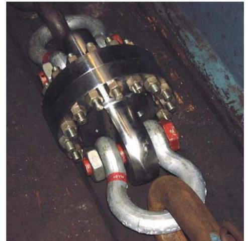
The bolting, if supplied without PTFE coating, should be lubricated with clean light oil, grease or proprietary anti-scuffing agent.
