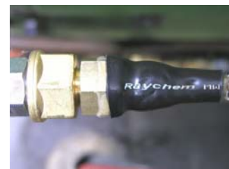
Photo 3 Protection with shrink tubing
